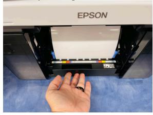
17. Replace the waste paper tray by aligning the tabs on the bottom and then locking it in place at the top.
