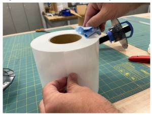
10. With the paper coming towards you over the back side of the roll, insert the right side of the spindle into the roll until it is fully inserted.
