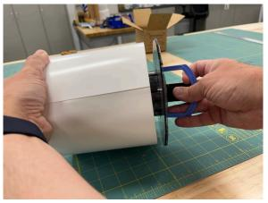
11. Using the cloth wipe the other edge of the roll to remove dust before adding the other end of the spindle onto the post.
