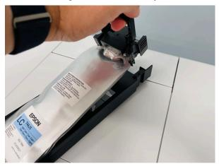
5. Aligning the groove in the sides of the cartridge with the tray, set the new tray in place.
