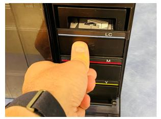
a. There is a specific set of slots in the front of the cartridge, if the wrong color is being put in the printer it will not fully load the tray.
