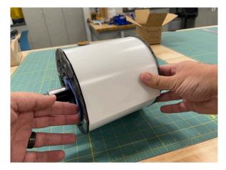
13. Set the spindle on the track so that the toothed gear aligns with the gear on the tray.
