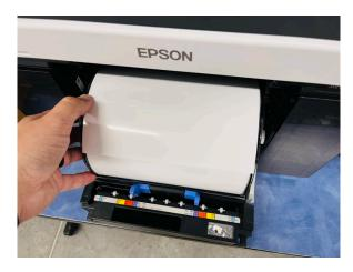
14. Take the paper and insert the end of the roll gently into the slot on the tray by the paper size gauge. Push it forward until the printer beeps.
