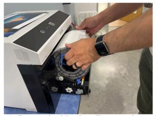
5. Set the roll on the table. Pull open the blue handles on either side and pull outwards to remove the spindle from the roll.
