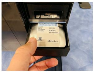
4. Using the handle, lift the old cartridge out of the tray.
