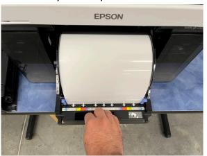
4. Carefully remove the roll from the tray by carrying from both sides of the roll.
