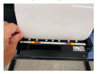
15. Adjust the guides on the sides of the tray to meet the edge of the paper.
