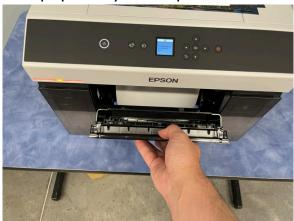
3. Slide the roll tray out from the body of the printer.
