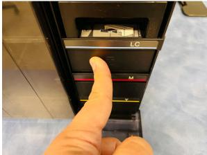
3. Remove the tray fully from the slot.
