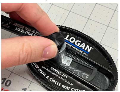
3. Slide the center post along the track inside the groove on the body of the cutter. Align the mark on the silver piece with the ruler to match the measurement you just found in step 1.
