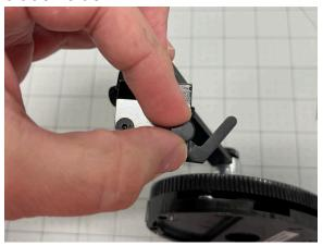
2. Insert the blade with the point facing the knob. Place it in until it stops moving. It should poke out the bottom just a small amount once in place.
