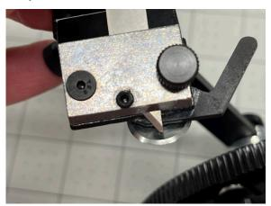
3. Tighten the knob to lock in the blade.
