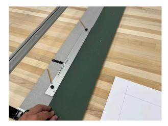
9. Lift the cover and insert the mat up to the right side of the gauge and along the bottom stop bar. Lower the cover.
