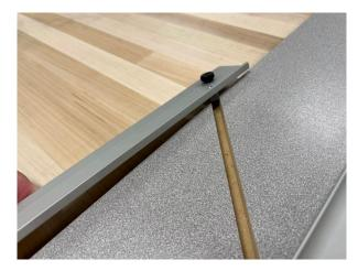
7. Align the left side of the scale with the distance you are cutting. Tighten the thumb screws to lock it in place.
