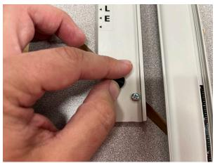
8. Insert the waste strip of mat board against the right side of the gauge.
