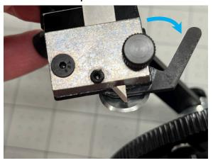
2. Align the points on the body of the cutter with the lines you drew on the mat. Press the cutter firmly into the mat to seat the pins on the underside into the mat board.
