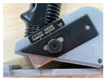
6. Align the groove on the right side of the cover with the slot on the cutter.
