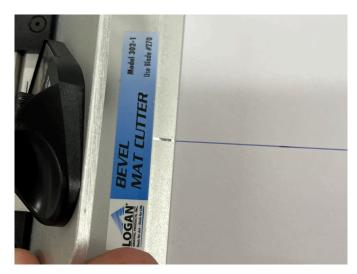
12. While firmly pressing down on the cover, press the blade in with your thumb and carefully push forward until the line on the bevel cutter is aligned with the top vertical line drawn on the mat. Release the blade and remove the bevel cutter.
