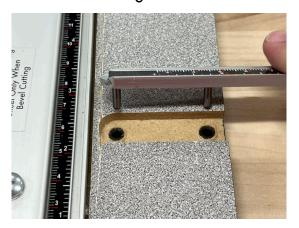
2. Loosen the thumb screw and slide the guide to the size you want to cut your mat to. Tighten the thumb screw.
