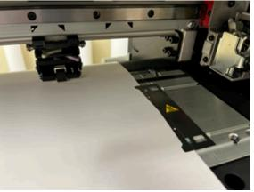
a. Note, for smaller rolls you may only use three pinch rollers, in which case the left most roller will not be on the media.
