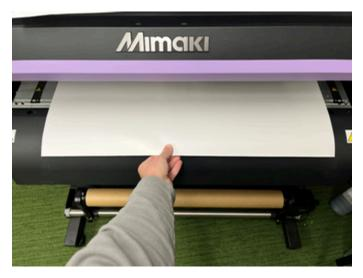
10. Place the hold downs over the left and right sides of the media and ensure that a pinch roller is sitting within the edge of your media.
