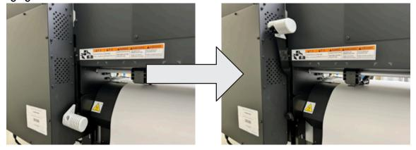
2. Wind the media on the machine back up and secure it with a Velcro strap.
