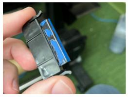
6. Take a cotton swab and clean out around and inside the spot where the wiper sits. Once it is cleaned, replace the wiper into the slot.
