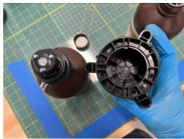
9. Twist the tightener until the red arrow reaches the green striped area. Do not overtighten past this point.
