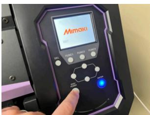
When attempting to turn off the machine, press and hold the End/Power button until it asks "Turn off Power? [ENT]" in which case you can press the Enter button to confirm.
