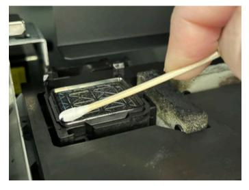
8. Once this is done you can pour any remaining cleaning solution left in the cap down the center of this. Pour slowly as it will overflow quickly. This will help flush old ink down into the waste bin.
