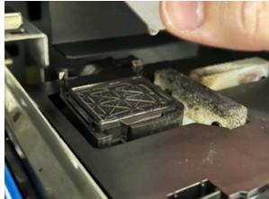
9. Replace the bottle and close all the doors, then press Enter on the printer to retract the head.
