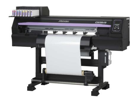
**Introduction:** The Mimaki Wide Format Printer/Cutter is a highly versatile tool that lets you print on large format rolls of media. Some of these options are also capable of being cut into custom shapes. The machine is currently equipped with six media types to allow you to create anything from stickers and window clings to banners and canvas prints.
