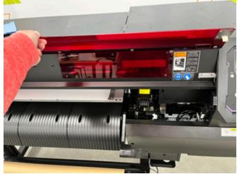
9. Return to the front of the machine. Grasp the media in the center of the roll. Gently pull forward until the media catches, then lightly wiggle the media left and right to ensure the roll is straight.
