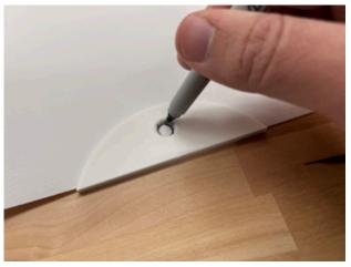
4. Align your mark with the post of the grommet press by slowly lowering the handle until you have aligned the two.
