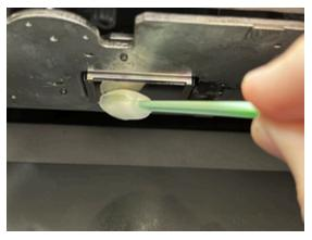
5. On the right hand side is a small blue wiper. Pinch both sides of it and remove the wiper from the machine. Using a cotton swab, dip it in the cleaning solution and proceed to clean all the used ink off of the wiper. It's important to get in all the cracks as best you can and get any dried ink out, not just off the blue part itself.
