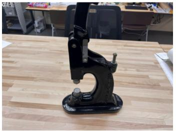
2. Take a bottom grommet piece with the rounded side down and put it in the lower die. Take the top piece and put it on the upper die with the rounded side up and the post facing down.
