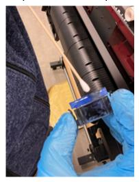
6. Take a cotton swab and clean out around and inside the spot where the wiper sits. Once it is cleaned, replace the wiper into the slot.
