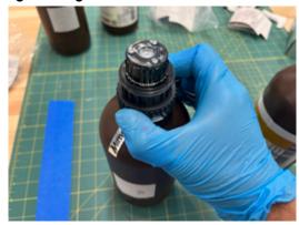
8. Using the cap tightener, align the pins with the slots in the tightener.
