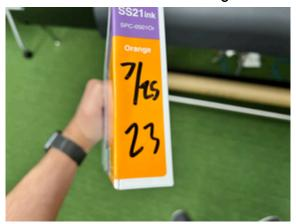
3. Remove the old ink cartridge from the machine by pulling outward until the entire cartridge is removed.
