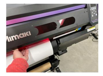
13. On the screen for the machine it will ask if you are using a roll or a leaf. If using a roll, press the left button.
