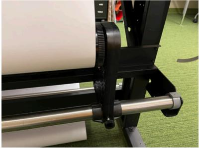
4. Take the new media roll and orient it so the edge of the media is coming from the bottom toward the back of the machine.
