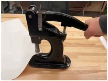
6. Release the handle. If your grommet was not pressed fully and is loose, realign the grommet to the dies and press it a second time until firmly closed. These are a little loose so don't think you need to get it completely snug.
