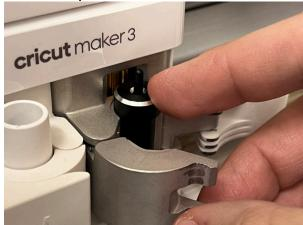
3. Close the clamp on side B to lock it in place.
