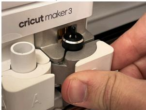
4. Some housings have a gear on the top of it. If so, align the gear with the teeth in the machine.
