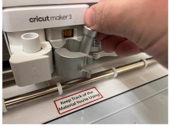
2. Take the new blade housing and insert it where the other was, with the outer edge of the housing sitting on top of the clamp area.
