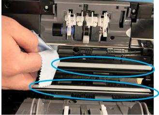
3. Using a cotton swab, locate the four sensors and gently remove any dust.
