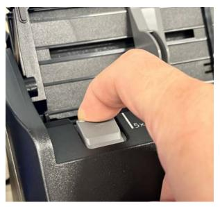
2. This opens the scanner and any jammed images can be removed.
