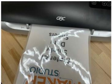
8. When the laminated document stops moving through the machine it's ready to remove.
