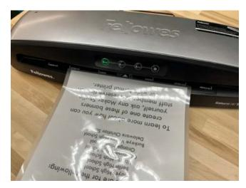
7. When the laminated document stops moving through the machine it's ready to remove.
