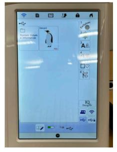
4. It is rare, but if the machine displays this error message, you can hit OK and move on. It refers to the Hatch software not providing a color code the machine can recognize. This may mean some of your colors look different. Remember the color of the thread is what determines the color in your design, not what is displayed on the screen.
