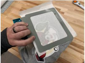
5. Insert the hoop into the machine. Be careful when guiding the material under the foot while inserting.
