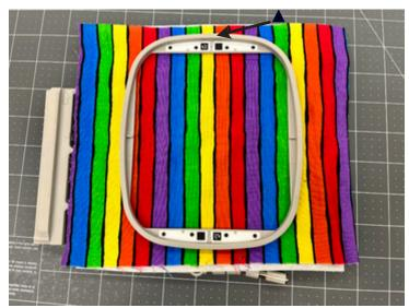
6. Press in the inner frame until it is seated fully inside the outer frame. You may need to loosen the thumb screw further to achieve this.
