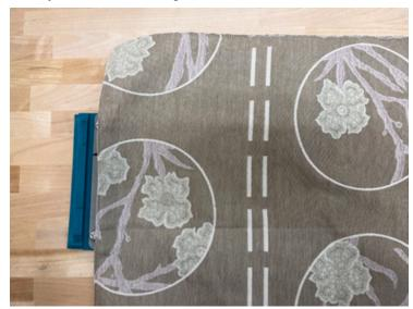
5. Set the top frame so that the rulers are facing up. It's best to align one edge of it before laying it down. Be careful not to catch your fingers inside the frame as the magnets are quite strong.
