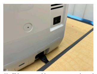
2. Switch the machine on. You'll be greeted by a message about the embroidery unit moving. Tap OK and wait for the machine to come to a rest. To do this, any hoops must be removed.
