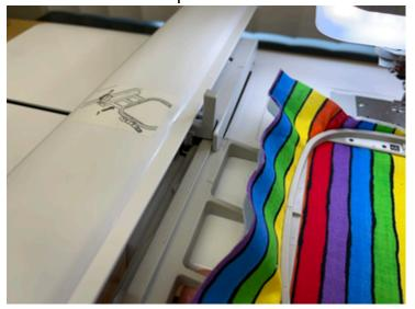
2. Once it is fully inserted, flip the locking lever down.
