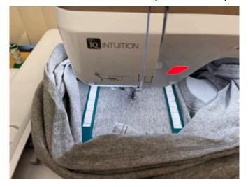
7. Ensure that no material is under the hoop on all sides.
