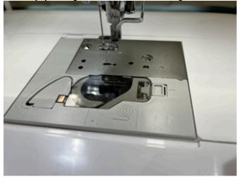
2. Drop the bobbin in with the thread running counter clockwise.
