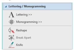
When adding text to your design you have two options. Lettering lets you type specific text onto the screen and adjust how it is laid out. Monogramming will use an initial design and modify it with additional elements. We'll look first at lettering.
