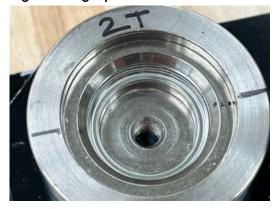
2. Rotate the dies 180 degrees and press the handle down to the left once again. Release the handle to the right and rotate the dies out to retrieve your pressed button shell.
