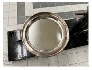
2. Rotate the dies 180 degrees and press the handle down to the left once again. Release the handle to the right and rotate the dies out to retrieve your pressed magnet shell.
