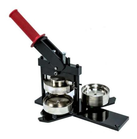
**Introduction:** The Maker Studio has two sizes of button maker, 1.25" and 3". Each of these is equipped to make the buttons with a pin back or a magnetic back. The 1.25" can also be turned into a keychain and the 3" can support a magnetic badge finding.
