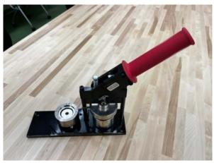
3. Rotate the center dies until you see the side labeled 1. Set that all the way on the left side so the dies are locked in place.
