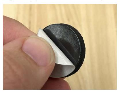
4. Place the magnet into the shell with the sticky side inside the shell. Press firmly to adhere the sticky side to the shell.
