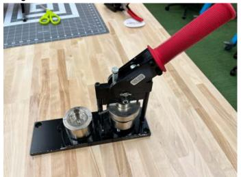
8. Press the three pieces together by rotating the handle to the left all the way. Then you can return the handle back to the right. These pieces are now held together in the top die.
