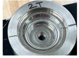
2. Rotate the dies 180 degrees and press the handle down to the left once again. Release the handle to the right and rotate the dies out to retrieve your pressed magnet shell.
