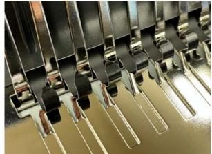
4. Place your front cover face down onto the combs. Repeat this process with batches of punched sheets until all the pages have been added to the comb.
