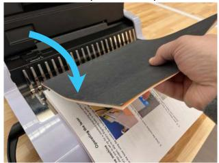
5. Place the back cover on last and fully return the handle back to close the comb.
