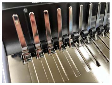
3. Pull forward on the left handle slowly, just enough to to open the comb and expose the teeth. Don't pull the handle too far or else you could launch the comb out of the machine.
