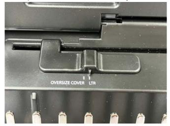
2. Take a bundle of no more than 20 sheets of paper and place them into this slot so that they are right next to the arm on the back of the switch. Note that the thickness of the paper will determine the actual quantity and you may not be able to fit the full 20 sheets in at once.
